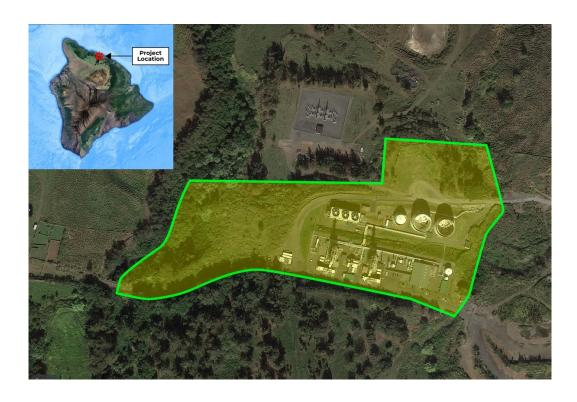
The "green outline" reflects the current TMK location. This current site at Honokaa, Hawaii, hosts a 60 MW combined cycle plant with two combustion turbines and one steam turbine. The current combined cycle plant has been in operation since 2000, providing 60MWs of capacity to the Island of Hawaii for over 20 years.
